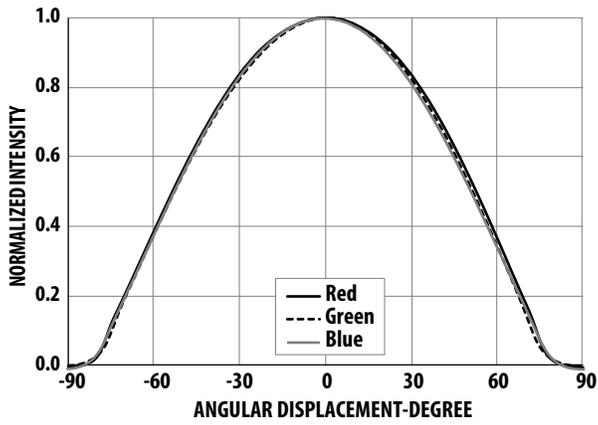
Figure 12 Radiation Pattern Along Y-Axis of the Package
