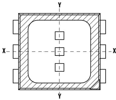
**Figure 14 Recommended Soldering Land Pattern**
