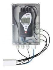
IP65 protection case with Multilogger holder and transparent lid. The case is equipped with cable glands for all Multilogger signals. Dimensions 190 x 280 x 95 mm.
