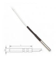
Multi-purpose watertight IP67 probe -190 to  $+150^{\circ}$ C. Accuracy class B. Stainless steel 17240 with teflon cable of specified length, without connector. Diameter 5  $\pm$  0.1 mm, length 50mm.
