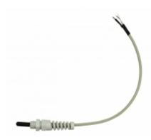
Precise IP67 watertight probe -30 to  $+80^{\circ}$ C for use in COMETEO solar radiation shields F8100 and F8200.
