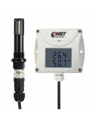
Humidity, temperature transmitter. T+RH probe from hard anodized duralumin for compressed air up to 25 bars on the cable. Humidity, temperature probe on a cable. Measured values are also converted to other humidity interpretation: dew point temperature, absolute humidity, specific humidity, mixing ratio, specific enthalpy.
