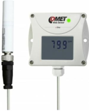
A multiple point CO<sub>2</sub> and temperature adjustment procedure leads to excellent CO<sub>2</sub> measurement accuracy over the entire temperature working range; this is a must for process control and outdoor applications. The dual wavelength NDIR CO<sub>2</sub> sensing procedure compensates automatically for ageing effects. The CO<sub>2</sub> module is highly resistant to pollution and offers maintenance free operation and outstanding long term stability.
