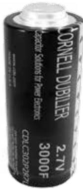
This leading edge large cell ultracapacitor, with low RC time constants, offers flexible mounting with two M6 thread holes on each end in weldable terminals. They are especially suited for back-up and pulse power applications such as grid stabilization and wind turbine pitch control. When assembled into modules, the low connection resistance design excels in transportation applications like automotive subsystems, rail system power and utility vehicles.
