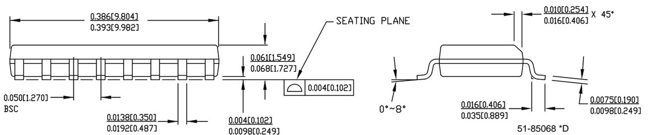
Figure 12. 16-Pin TSSOP 4.40 MM Body Z16.173
