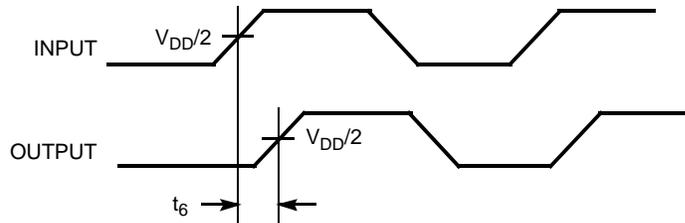
Figure 8. Device-Device Skew
