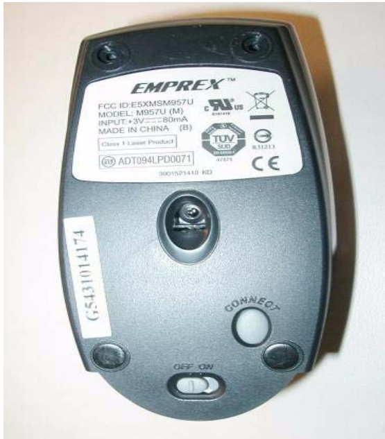
Figure 3-1. Bottom View Bind Button and On-Off Switch
