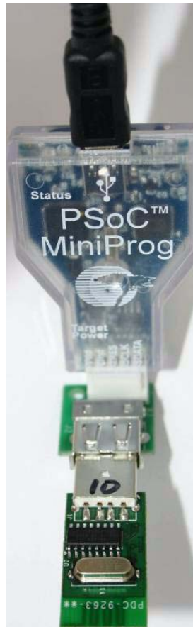
Figure 5-4. RDK Bridge with USB Adapter and PSoC MiniProg
