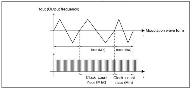
MB88152A contains the modulation period to realize the efficient EMI reduction.
