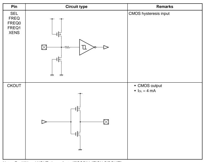
Note: For XIN and XOUT pins, refer to "■OSCILLATION CIRCUIT".
