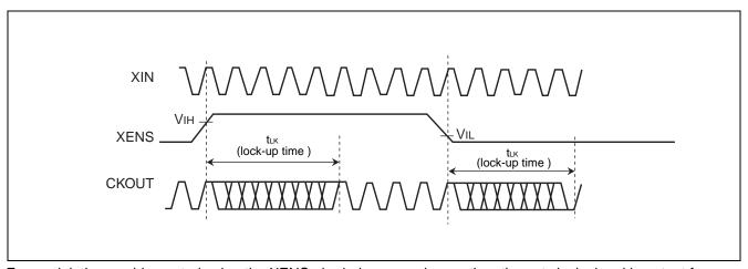
For modulation enable control using the XENS pin during normal operation, the set clock signal is output from CKOUT pin at most the lock-up time ( $t_{LK}$ ) after the level at the XENS pin is determined.
