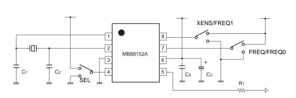
C<sub>1</sub>, C<sub>2</sub> : Oscillation stabilization capacitance (refer to "■ OSCILLATION CIRCUIT".)
