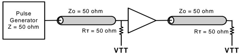
**Figure 3. Propagation Delay  $t(\phi)$ , Static Phase Offset**
