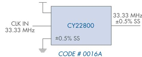
To generate your PCI frequency with or without spread spectrum (SS), use Jedec code #0011A and #0016A, respectively.
