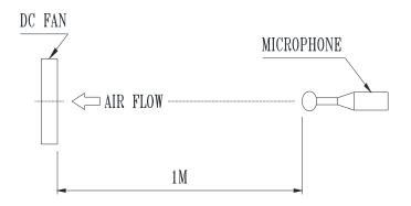
NOISE IS MEASURED AT RATED VOLTAGE IN FREE AIR IN SEMI-ANECHOIC CHAMBER WITH MICROPHONE AT A DISTANCE OF ONE METER FROM THE FAN INTAKE.
