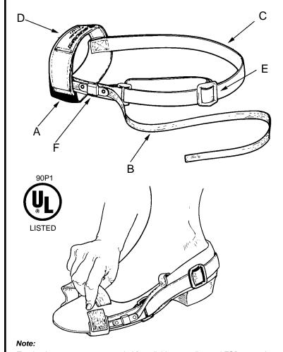
Two heel straps are recommended for reliable grounding and ESD protection. providing ground when one foot is off the floor.
