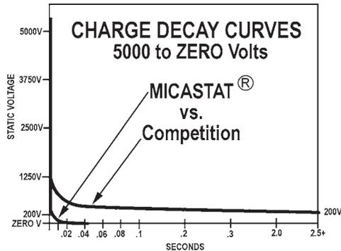
The premium choice for ESD bench dissipative worksurfaces. Provides a durable and attractive ESD controlled dissipative worksurface. Resists hot solder and most solvents; exceeds NEMA standards for wear resistance. Patented conductive layer provides superior charge dissipation and zero voltage suppression.
