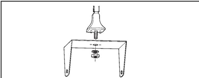
**Figure 4:** Installing The Extractor to Swing Arm
