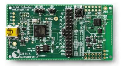
This Basic development kit gives you all flexibility to develop with confidence. All of the DA14581's I/Os are available and mapped on to expansion connectors. A debugger is provided on the PCB which in combination with SmartSnippets™, Dialog's complete software environment, enables you to program and test your A4WP or HCl application.
