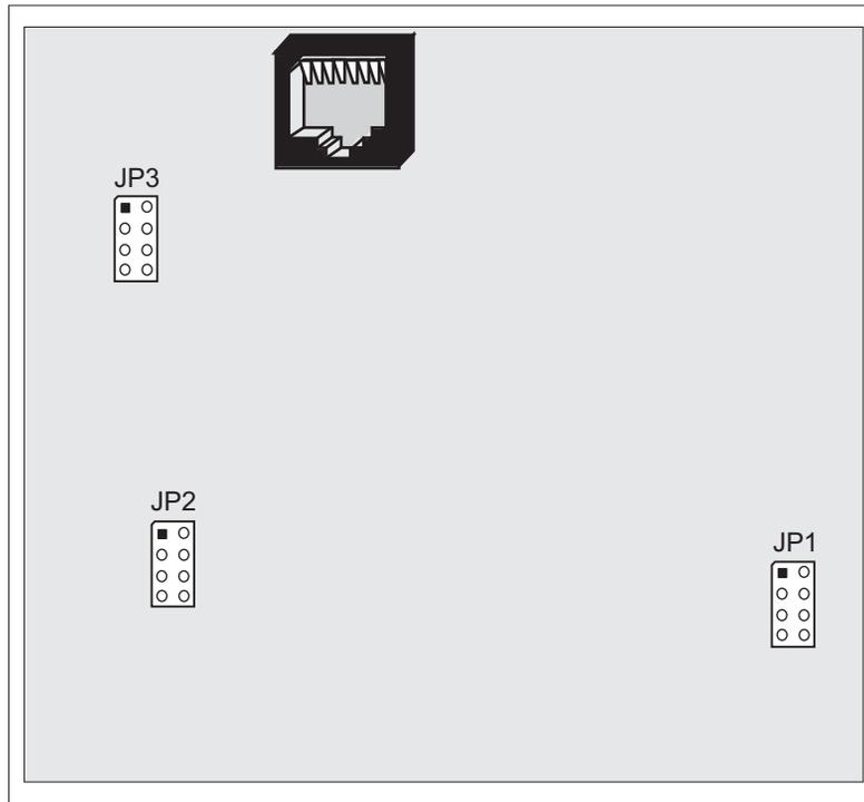
**Figure 16. Location of Digital I/O Card Configurable Positions**
