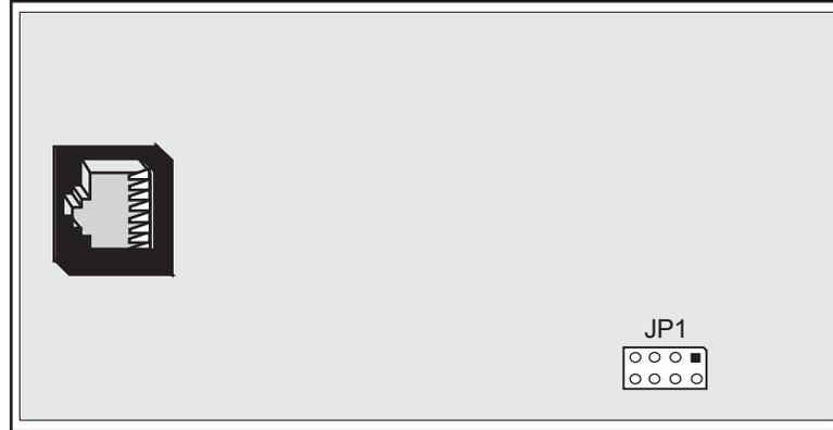
**Figure 26. Location of A/D Converter Card Configurable Positions**
