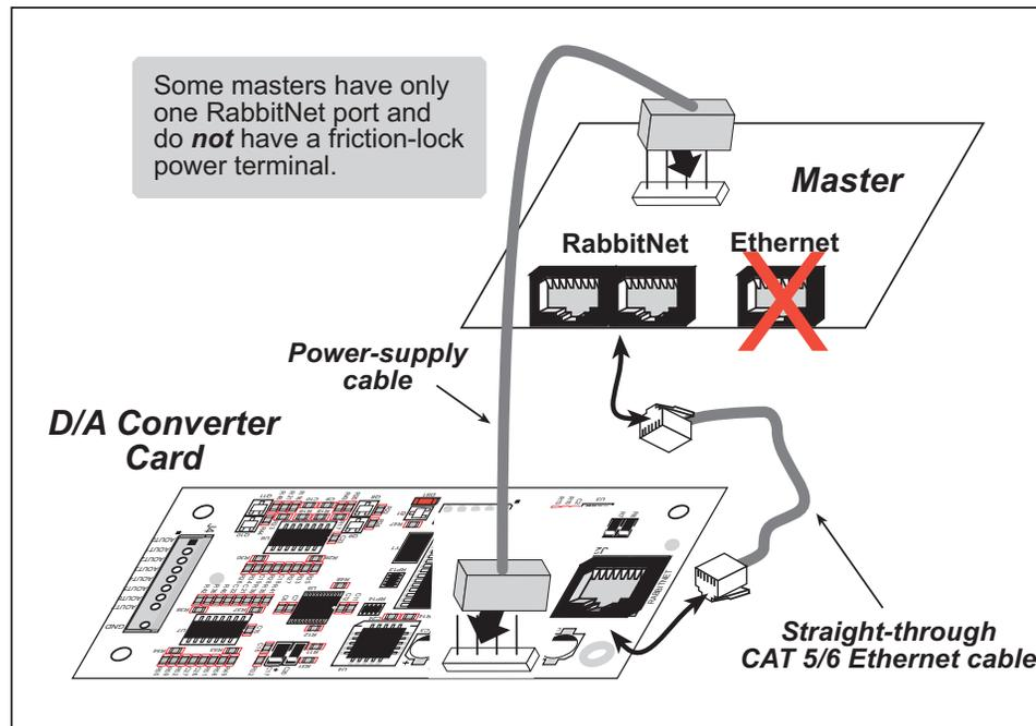
**Figure 28. Connect D/A Converter Card to Master**
