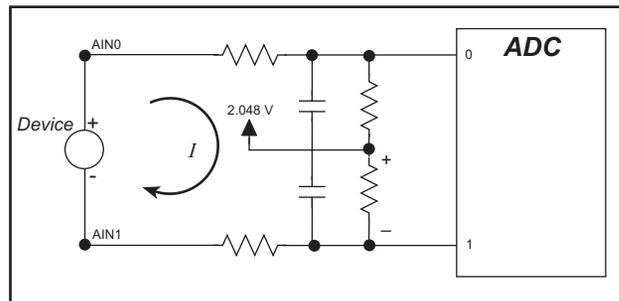
**Figure 22. Current Flow from Ungrounded or Floating Source**
