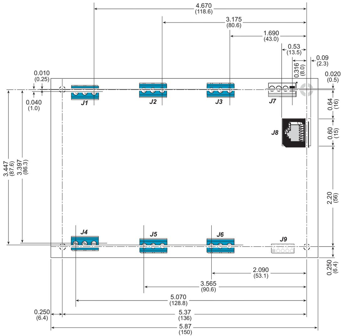
Figure 41. User Board Footprint for Relay Card
