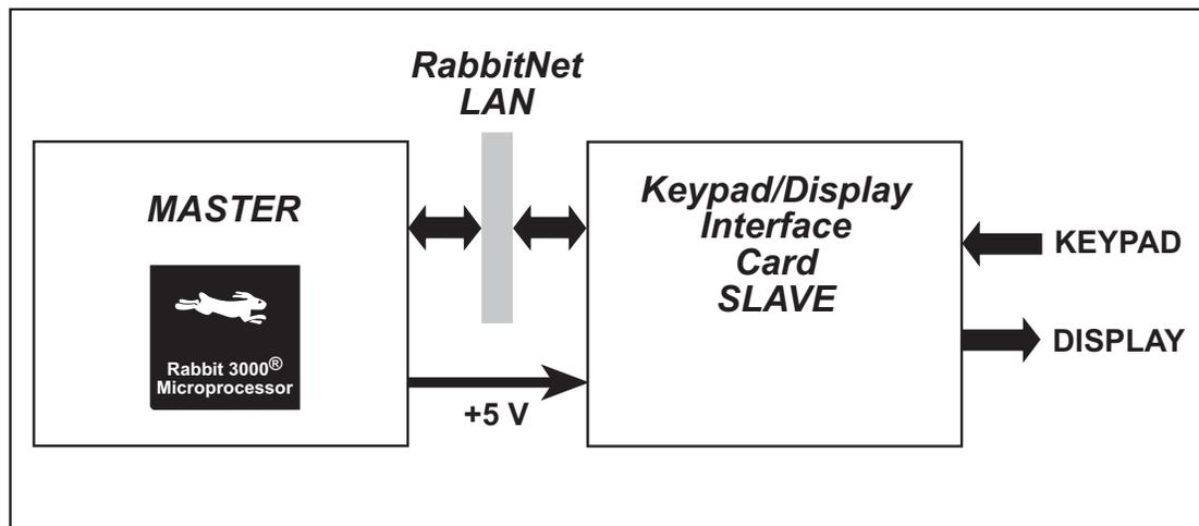
**Figure 42. RabbitNet Keypad/Display Interface (Slave) Connected to Master**
