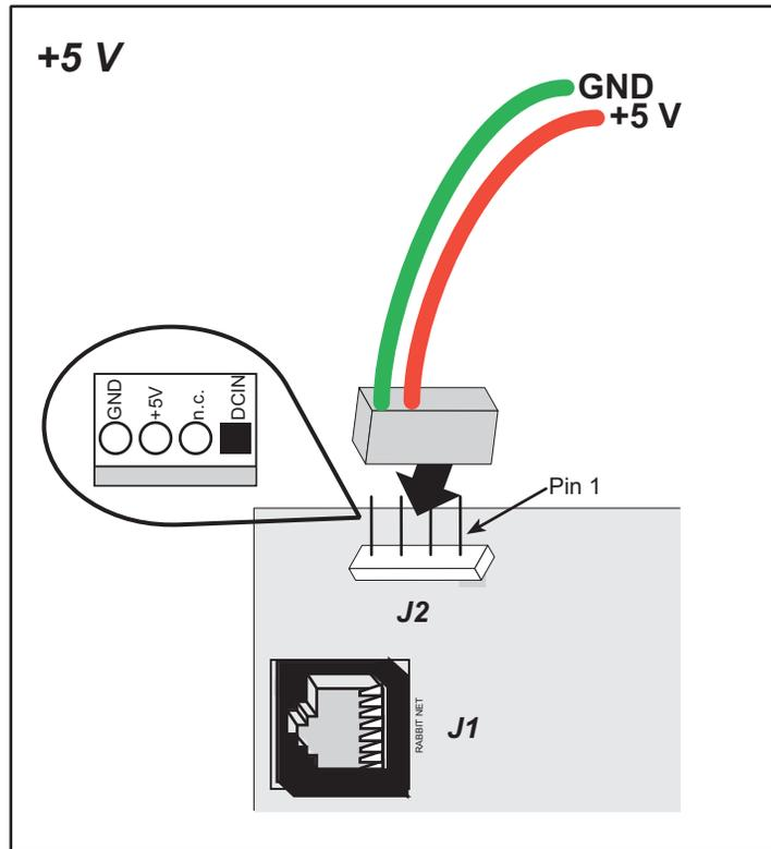
Figure 19. Power-Supply Connections
