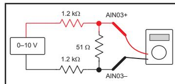
Now compile and run the sample program. Enter the voltage reading when prompted by the Dynamic C **STDIO** window. Then reverse the power supply + and – connections and hit the **Return** key in the Dynamic C **STDIO** window. Now enter the voltage reading again.
