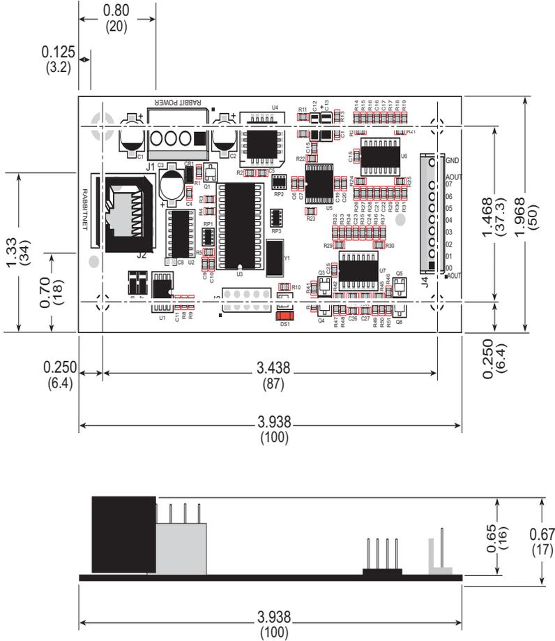
**Figure 32. D/A Converter Card Dimensions**
