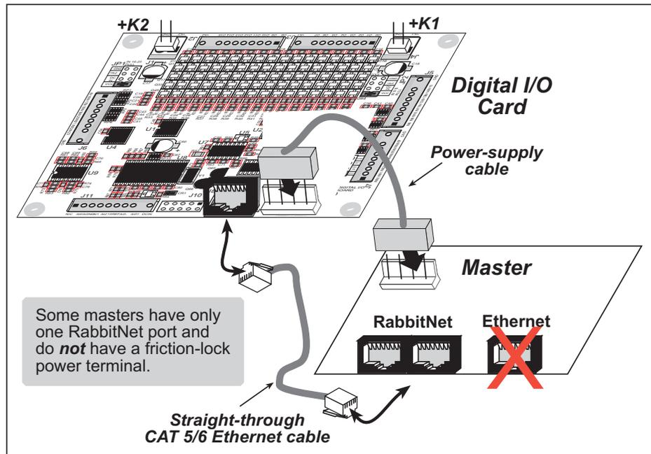
**Figure 4. Connect Digital I/O Card to Master**
