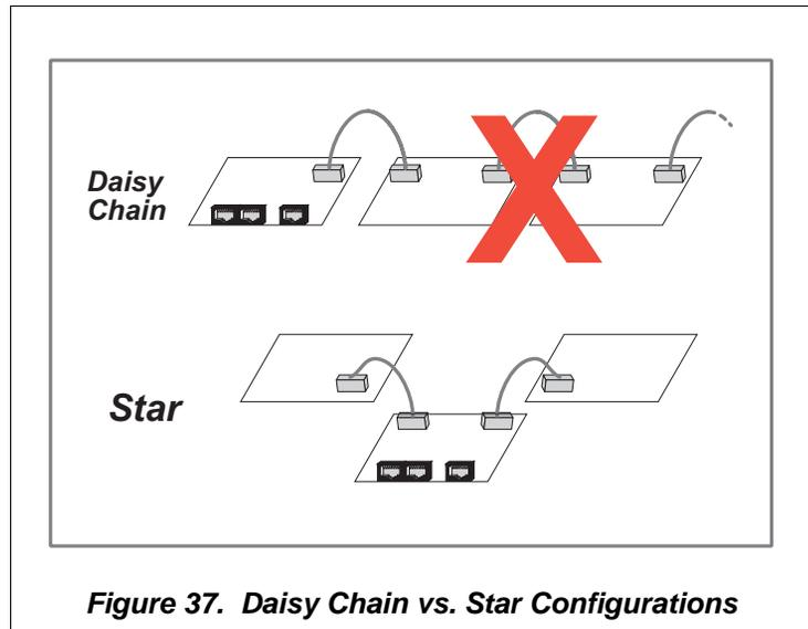
**Figure 37. Daisy Chain vs. Star Configurations**
