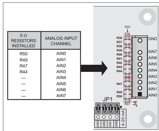
**Figure 23. Locations of Resistors for 4–20 mA Mode**
