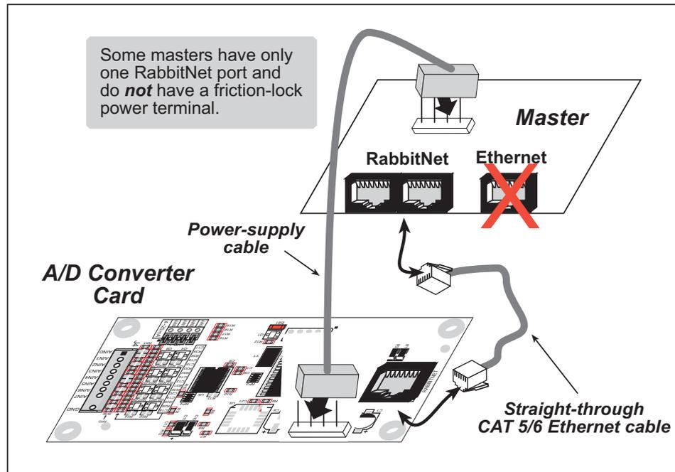
**Figure 18. Connect A/D Converter Card to Master**
