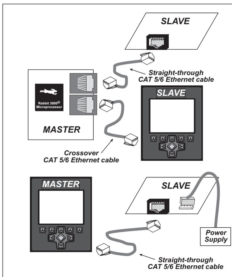
Figure 1. Connecting Peripheral Cards to a Master
