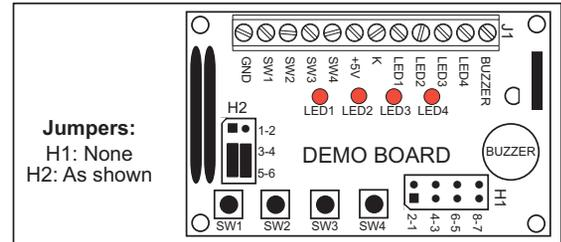
Once this sample program is compiled and running, you may press switches S1–S4 on the Demonstration Board to toggle the input low on the corresponding channel. Inputs IN04–IN23 can be toggled low by touching the line with a GND signal. The status of the inputs is displayed in the Dynamic C **STDIO** window.
