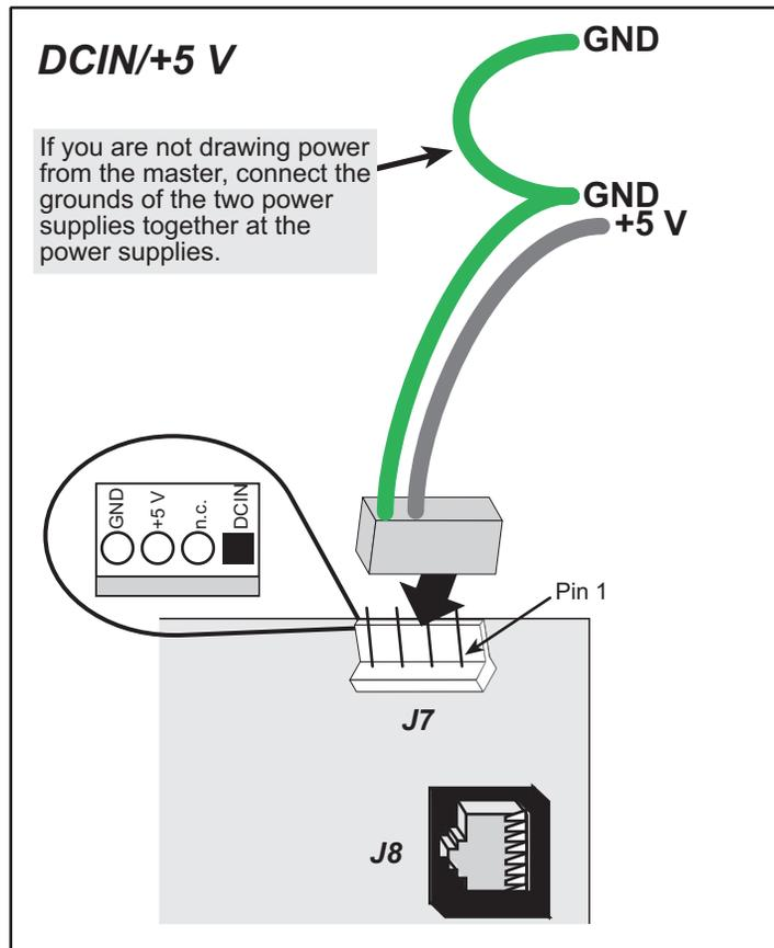
**Figure 36. Power-Supply Connections**
