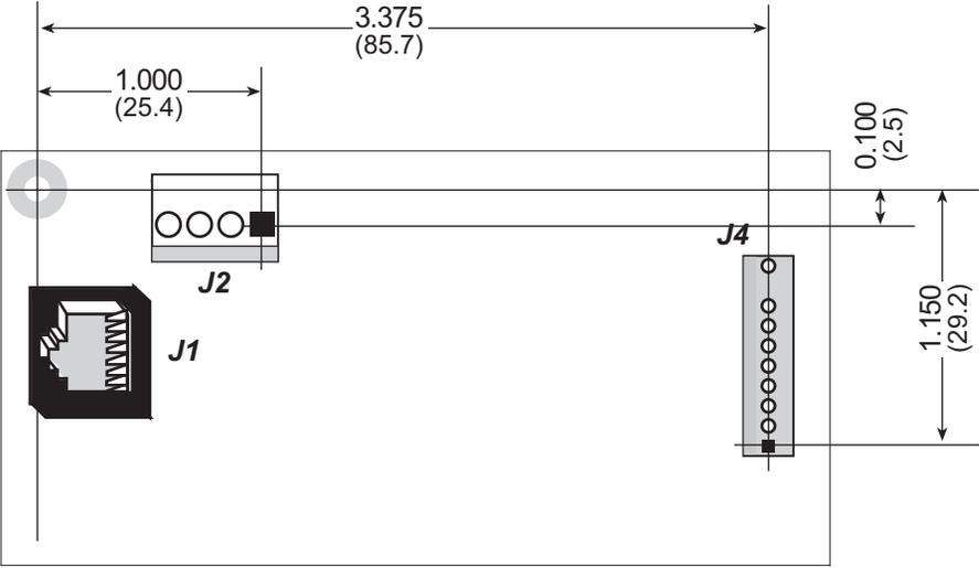
Figure 25. User Board Footprint for A/D Converter Card
