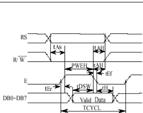
(WRITE DATA FROM MPU TO MODULE)
