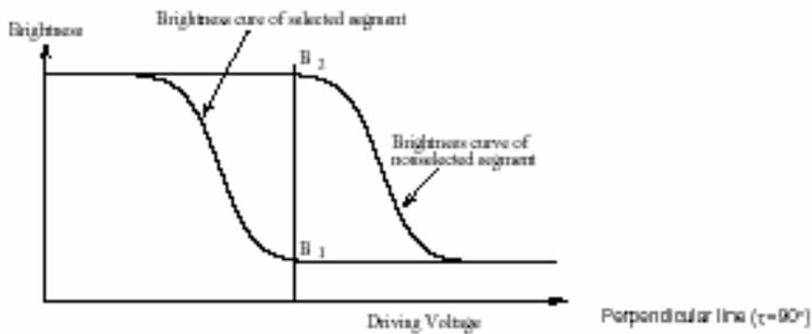
$$\text{Contrast ratio} = \frac{\text{Brightness at nonselected segment (B2)}}{\text{Brightness at selected segment (B1)}}$$
