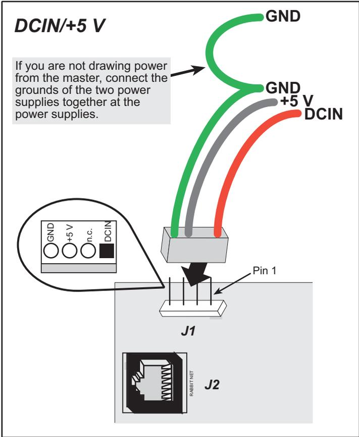
Figure 29. Power-Supply Connections
