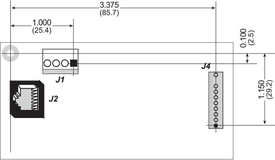
Figure 33. User Board Footprint for D/A Converter Card
