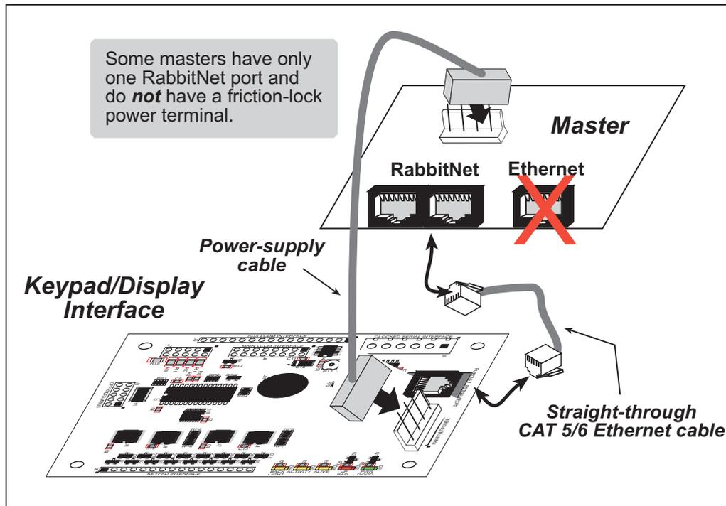
**Figure 43. Connect RabbitNet Keypad/Display Interface to Master**
