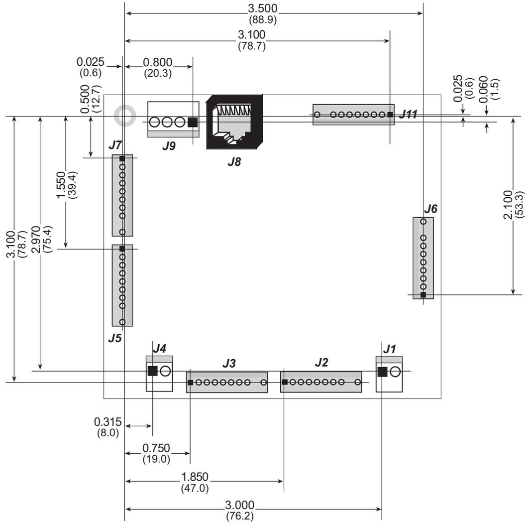
**Figure 15. User Board Footprint for Digital I/O Card**
