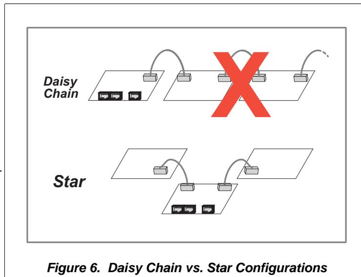
**Figure 6. Daisy Chain vs. Star Configurations**
