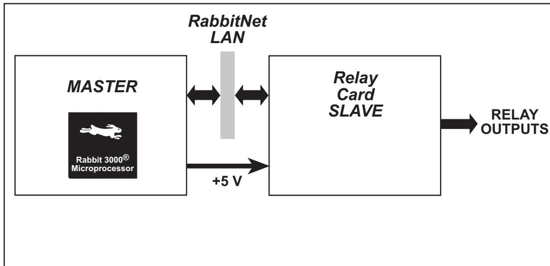
**Figure 34. Relay Card (Slave) Connected to Master**
