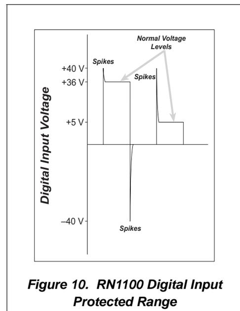
**Figure 10. RN1100 Digital Input Protected Range**
