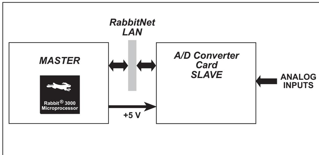
**Figure 17. A/D Converter Card (Slave) Connected to Master**
