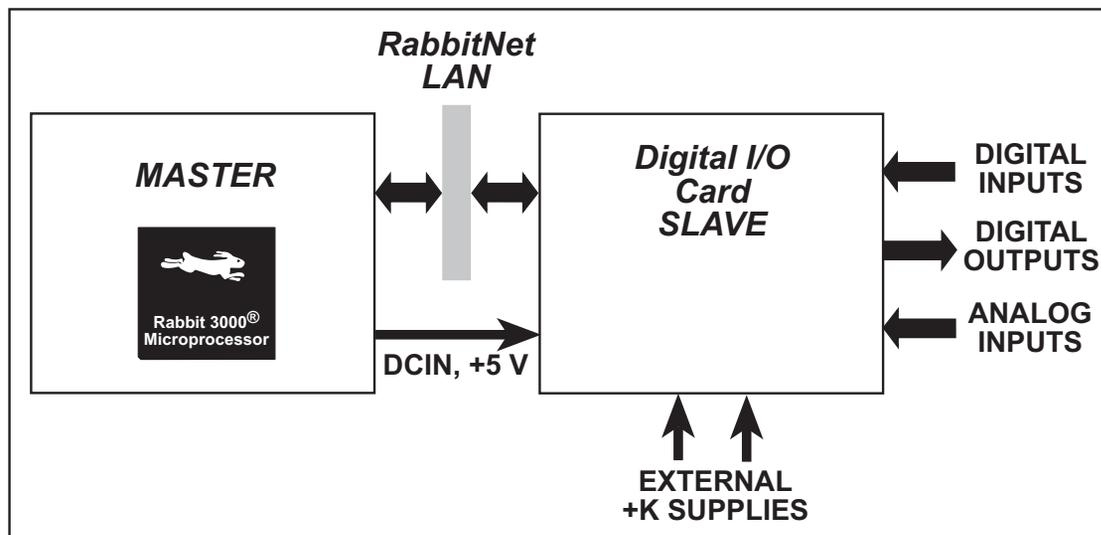
**Figure 3. Digital I/O Card (Slave) Connected to Master**
