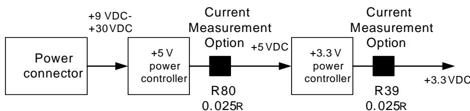
To measure the load current used on different power supplies, measure DC voltage across the sense (CMO) resistor. The value of the resistor is  $0.025\Omega \pm 1\%$ . Calculate the current using this equation:  $I = U/R$
