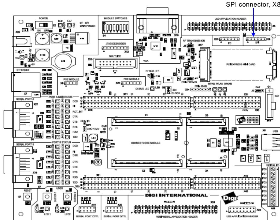
The development board provides access to the SPI interface on the module using the SPI connector, X8. Because the module's SPI interface is shared with a UART interface, you cannot use both simultaneously. The SPI interface on the development board is shared with UART\_B (NS9360 port B).
