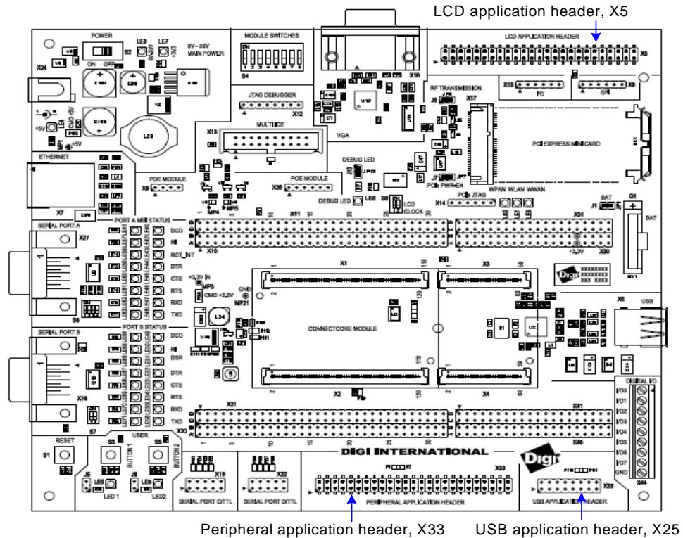
The development board provides two, 2x25-pin, 0.10" (2.54mm) pitch headers for supporting application-specific daughter cards/expansion boards:
