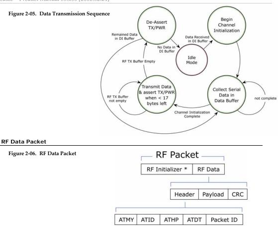
\* When streaming multiple RF packets, the RF Initializer is only sent in front of the first packet.
