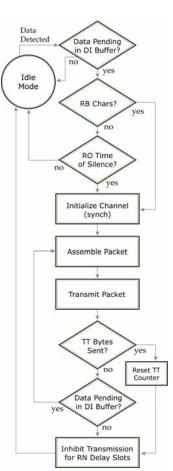
parameter is set to a non-zero value. These delays are intended to lessen congestion following long bursts of packets from a single transmitting module, during which several receiving modules may have become ready to transmit.
