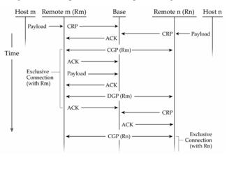
CRP = Connection Request Packet CGP = Connection Grant Packet DRP = Disconnect Request Packet (not shown in diagram – applicable when remote connection is disconnected using the pin sleep I/O line.
