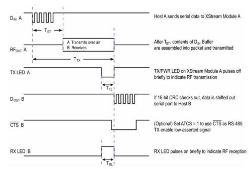
Figure 1-04. Timing Specifications ("A" and "B" refer to Figure 1-03.)
