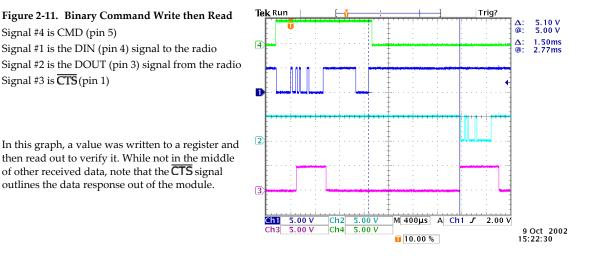
IMPORTANT:For the XStream Module to recognize a binary command, RT (DI2 Configuration)<br/>Command must be issued. If binary programming is not enabled ( $RT \neq 1$ ), the<br/>module will not recognize that the CMD pin (Pin 5) is asserted and therefore will not<br/>recognize the data as binary commands.
