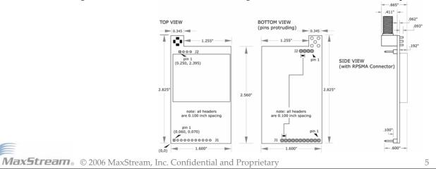
Figure 1-01. XStream Module Mechanical Drawings (shown with RPSMA antenna connector option)
