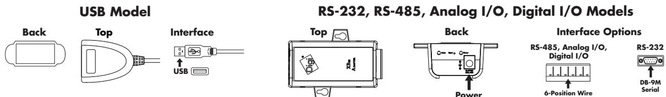
A complete list of models and part numbers is available at [www.digi.com/products/wireless/zigbee-mesh/xbee-zb-adapters.jsp](http://www.digi.com/products/wireless/zigbee-mesh/xbee-zb-adapters.jsp)
