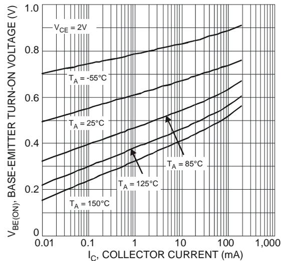
Fig. 7 Typical Base-Emitter Turn-On Voltage vs. Collector Current
