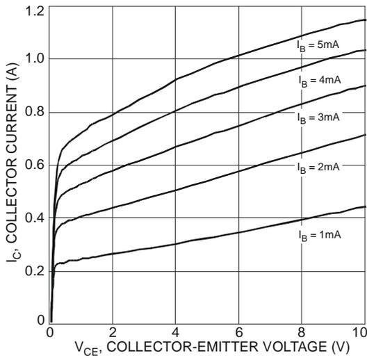
Fig. 4 Typical Collector Current vs. Collector-Emitter Voltage
