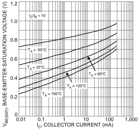
Fig. 10 Typical Base-Emitter Saturation Voltage vs. Collector Current
