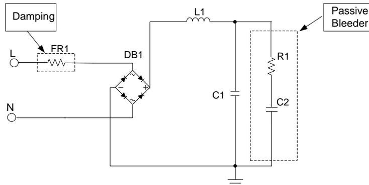
Figure 4 LED Driver Schematic with Passive Bleeder
