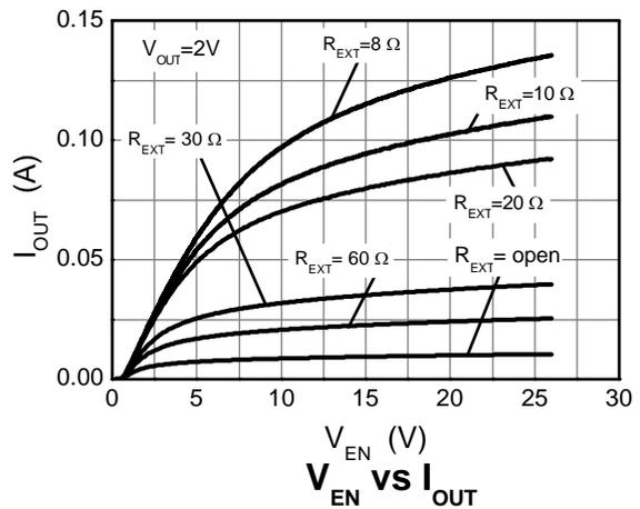
**Typical Electrical Characteristics BCR420U** (Cont.) (@T<sub>A</sub> = +25°C, unless otherwise specified.)
