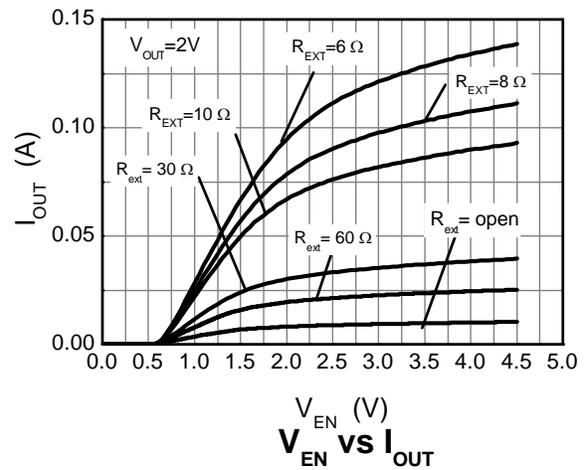
**Typical Electrical Characteristics BCR421U** (Cont.) (@T<sub>A</sub> = +25°C, unless otherwise specified.)
