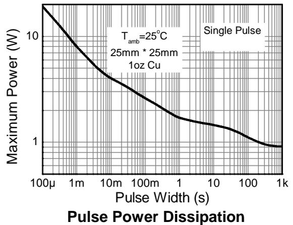
**Typical Electrical Characteristics BCR421U** (Cont.) (@T<sub>A</sub> = +25°C, unless otherwise specified.)
