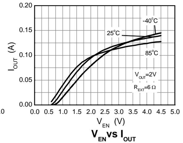
**Typical Electrical Characteristics BCR420U** (Cont.) (@ $T_A = +25^\circ\text{C}$ , unless otherwise specified.)
