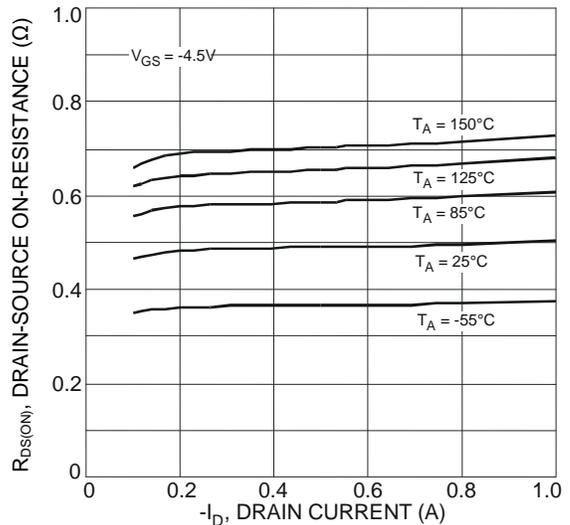
Fig. 14 Typical On-Resistance vs. Drain Current and Temperature
