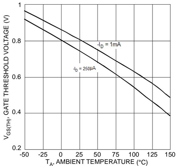
Figure 5 Gate Threshold Variation vs. Ambient Temperature
