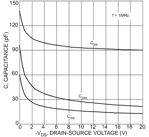
Figure 10 Typical Capacitance
