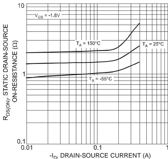
Figure 5 Static Drain-Source On-Resistance vs. Drain Current
