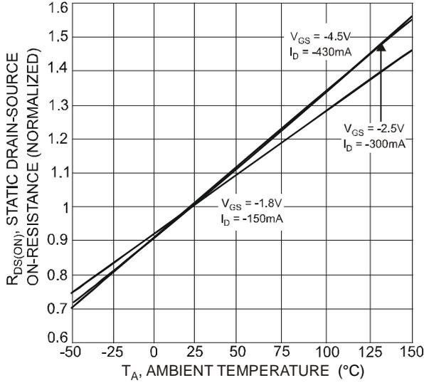
Figure 7 Static Drain-Source On-State Resistance vs. Ambient Temperature
