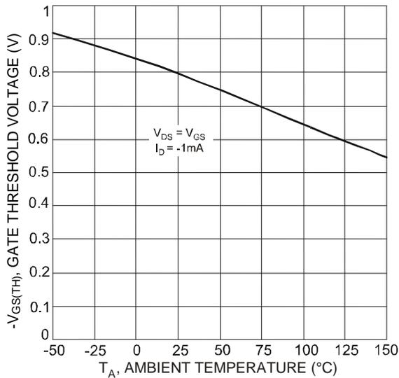
Figure 3 Gate Threshold Voltage vs. Ambient Temperature
