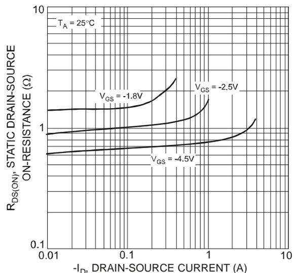
Figure 6 Static Drain-Source On-Resistance vs. Drain-Source Current
