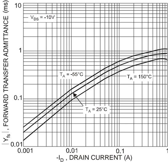
Figure 9 Forward Transfer Admittance vs. Drain Current
