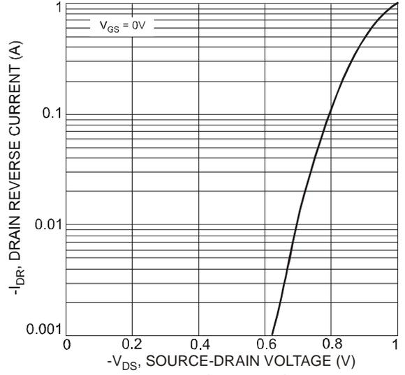
Figure 8 Reverse Drain Current vs. Source-Drain Voltage
