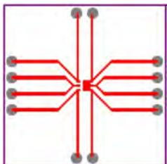
Notes: 5. Device mounted on FR-4 substrate PC board, 2oz copper, with thermal vias to bottom layer 1inch square copper plate
