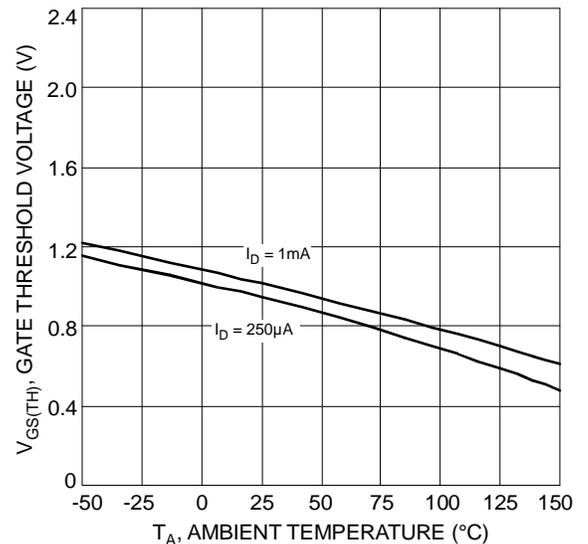
Fig. 6 Gate Threshold Variation vs. Ambient Temperature
