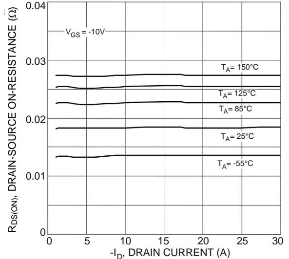
Figure 6 Typical On-Resistance vs. Drain Current and Temperature
