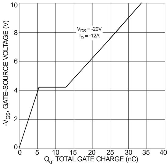
Figure 13 Gate-Charge Characteristics
