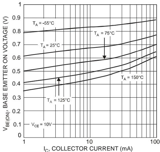
Fig. 5, Base-Emitter On Voltage vs. Collector Current
