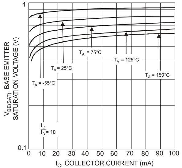
Fig. 4, Base Emitter Saturation Voltage vs. Collector Current
