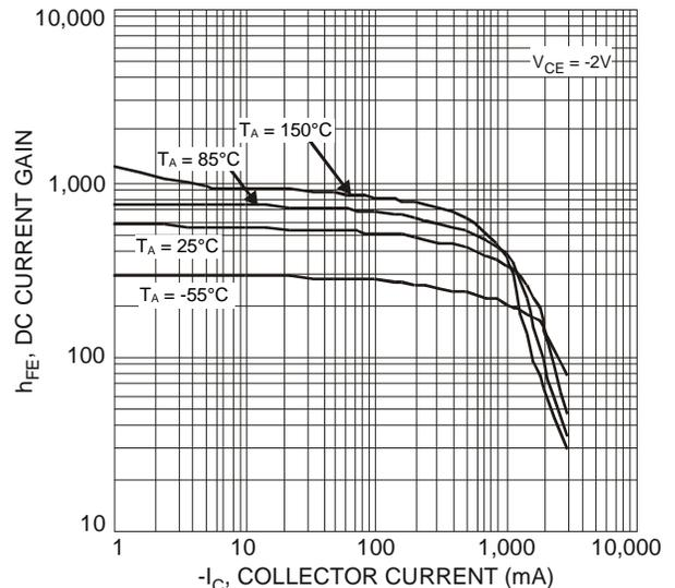
Figure 2 Typical DC Current Gain vs. Collector Current
