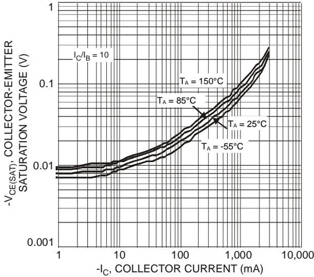
Figure 3 Typical Collector-Emitter Saturation Voltage vs. Collector Current
