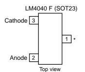
\* Pin 1 must be left floating or connected to pin 2
