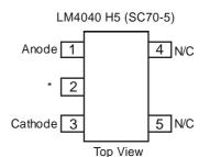
\* Pin 2 must be left floating or connected to pin 1
