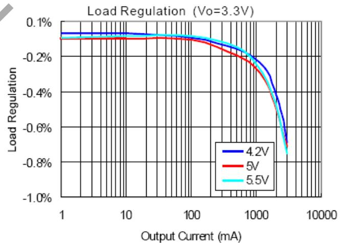
**Typical Performance Characteristics** (continued) (@T<sub>A</sub> = +25°C, C<sub>IN</sub> = 33μF, C<sub>O</sub> = 22μF, unless otherwise specified.)
