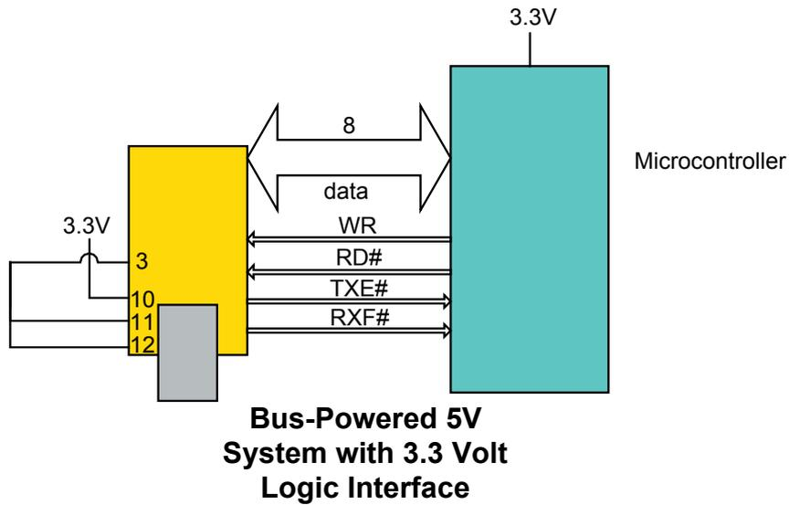
Figure 3 shows how to configure the DLP-USB245M to interface with a 3.3v logic device. In this example, the target electronics provides the 3.3 volts via the VCCIO line (pin 10) which in turn will cause the FIFO interface IO pins to drive out at 3.3v level.
