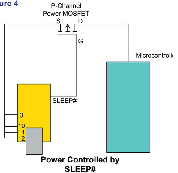
recommend that a dedicated power switch i.c with inbuilt “soft-start” is used instead of a MOSFET. A suitable power switch i.c. for such an application would be a Micrel ([www.micrel.com](http://www.micrel.com)) MIC2025-2BM or equivalent.
