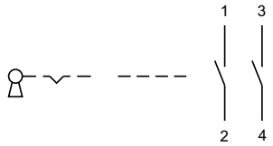
72 Keylock switch 2 positions page 9 | Keylock switch actuator 2 positions, flush mounting page 15
