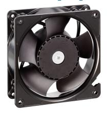
119 mm mixed flow fan with very high air performance. The DC drive employs an electronically commutated external rotor motor with high efficiency. Drive electronics is completely integrated into the fan hub.
