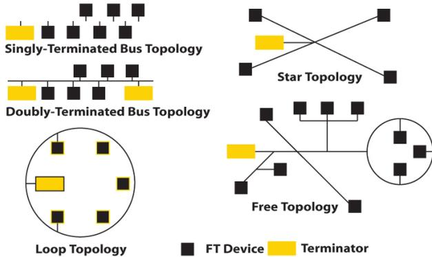
**Figure 2: FT Free Topology Network Configurations**
