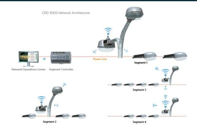
3000installs in existing ANSI compliant pole top sockets. The CRD 3000 installs without software tools, using simple, on/off indicator lights to tell installers that reliable RF communications have been established within seconds of installation. As an integral infrastructure device, no changes are required to existing maintenance, management, and visualization software for LonWorks based street lighting networks utilizing the SLB.
