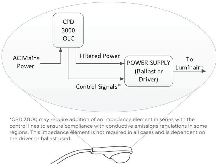
\*CPD 3000 may require addition of an impedance element in series with the control lines to ensure compliance with conductive emissions regulations in some regions. This impedance element is not required in all cases and is dependent on the driver or ballast used.
