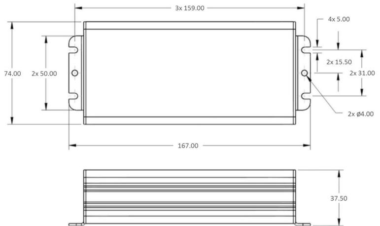
**Figure 3. CPD 3000 Housing Profile (dimensions in millimeters)**
