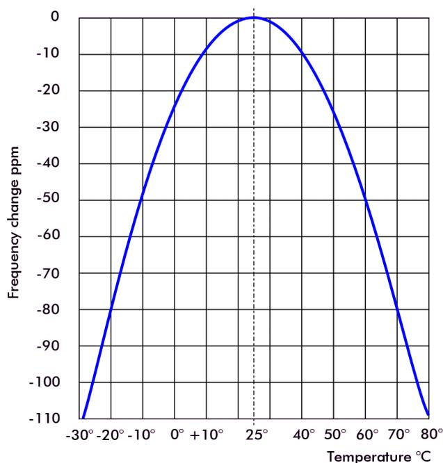
$$\text{Function} = \Delta f / f_0 = -0.035(T - T_0)^2 \pm 10\%$$
