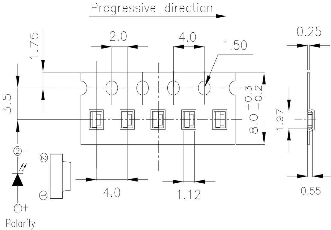
Note: The tolerances unless mentioned is  $\pm 0.1\text{mm}$ , Unit = mm
