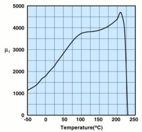
Measured on an 18/10/6mm toroid at 100kHz.
