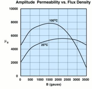
Measured on an 18/10/6mm toroid at 10kHz.
