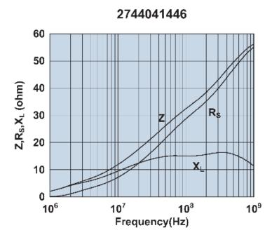
Impedance, reactance, and resistance vs. frequency.
