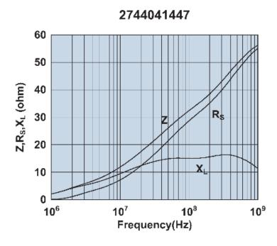
Impedance, reactance, and resistance vs. frequency.
