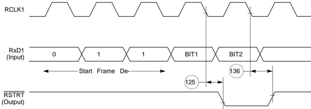
Figure 61. CAM Interface Receive Start Timing Diagram
