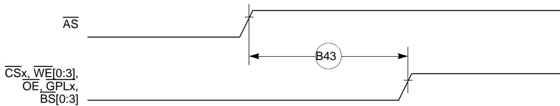
**Figure 21. Asynchronous External Master—Control Signals Negation Timing**
