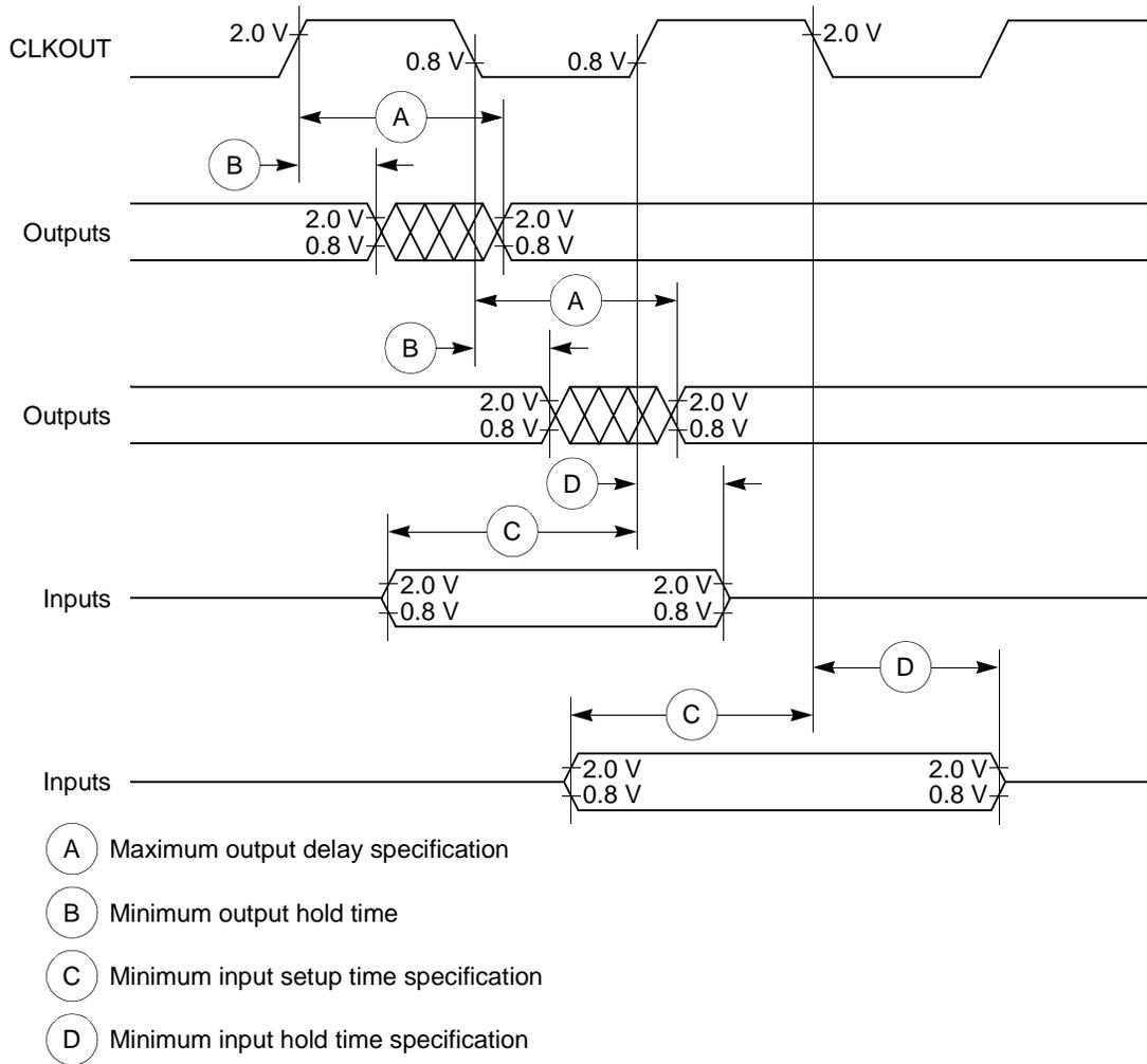
**Figure 2. Control Timing**
