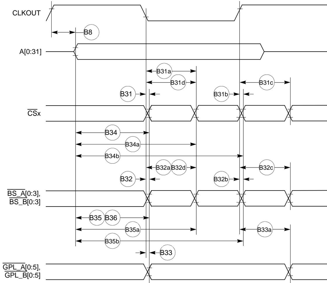
Figure 16. External Bus Timing (UPM Controlled Signals)
