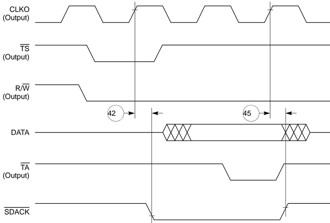
Figure 47.  $\overline{\text{SDACK}}$  Timing Diagram—Peripheral Read, Internally-Generated  $\overline{\text{TA}}$
