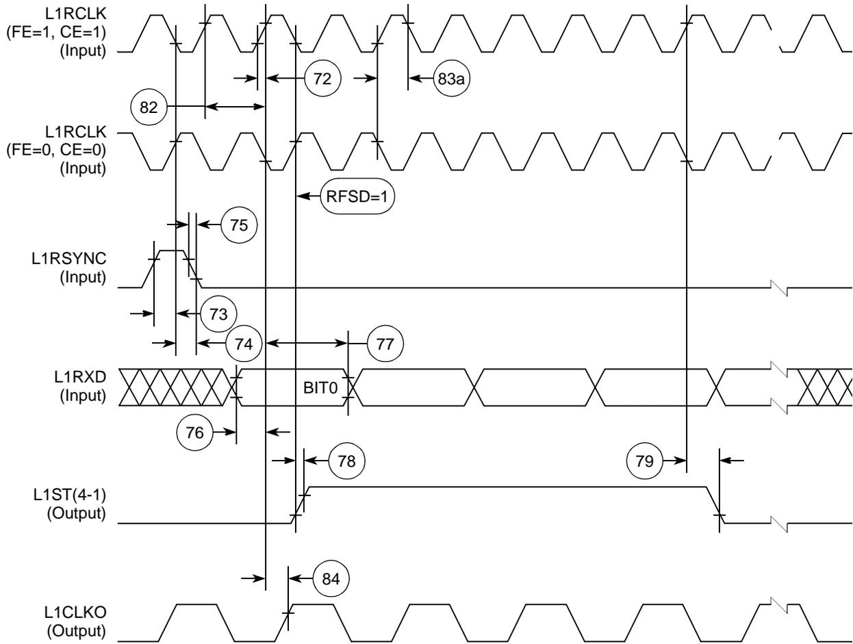
Figure 51. SI Receive Timing with Double-Speed Clocking (DSC = 1)
