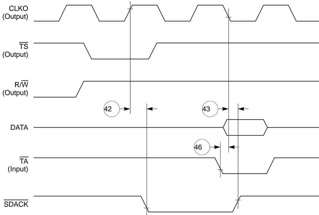
Figure 45.  $\overline{\text{SDACK}}$  Timing Diagram—Peripheral Write, Externally-Generated  $\overline{\text{TA}}$
