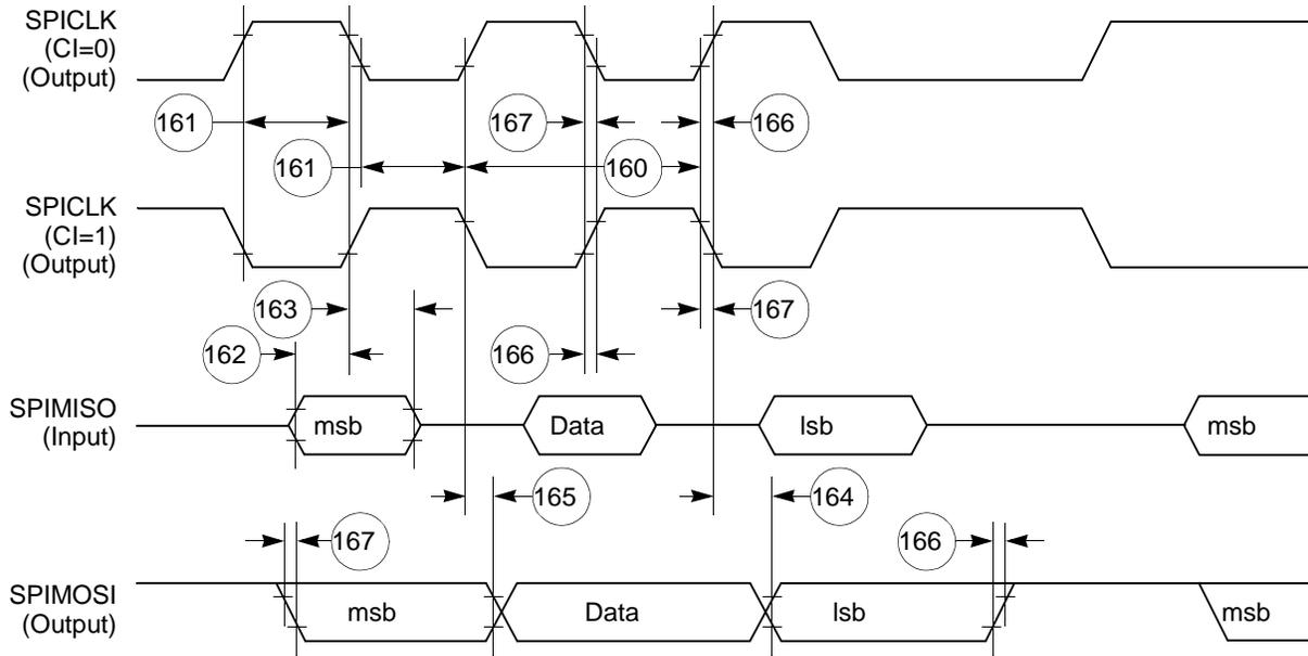
Figure 65. SPI Master (CP = 1) Timing Diagram
