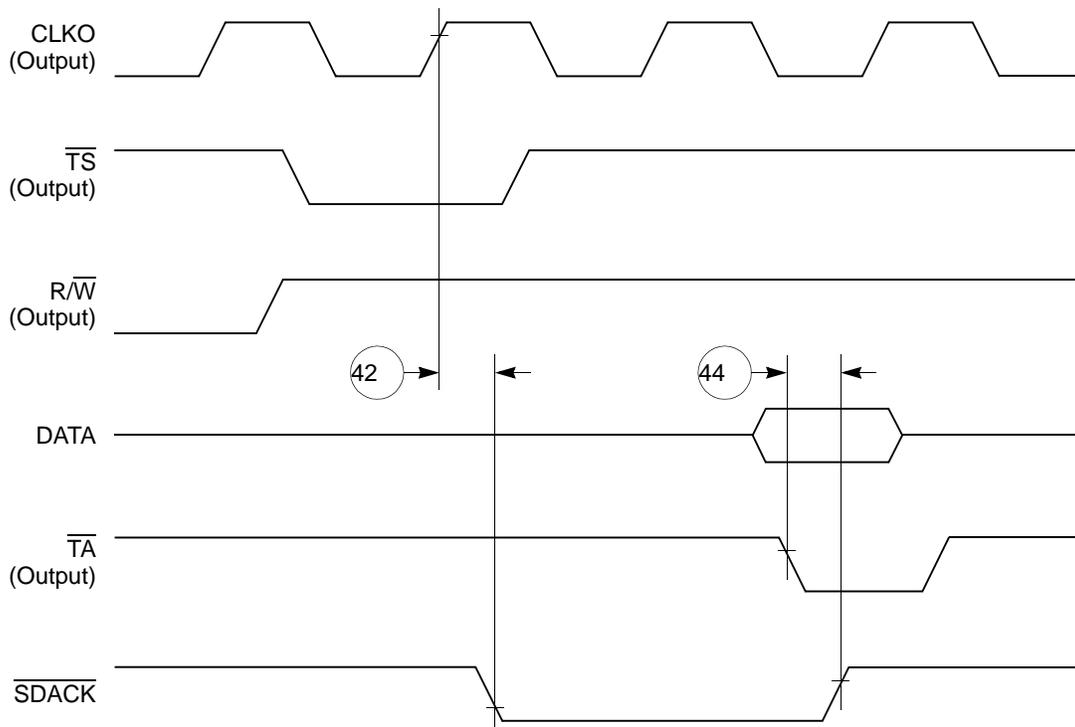
Figure 46.  $\overline{\text{SDACK}}$  Timing Diagram—Peripheral Write, Internally-Generated  $\overline{\text{TA}}$
