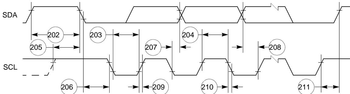
Figure 68. I<sup>2</sup>C Bus Timing Diagram
