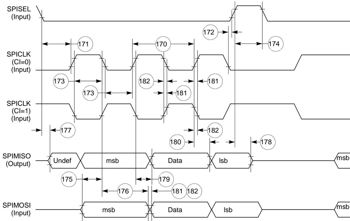
Figure 67. SPI Slave (CP = 1) Timing Diagram
