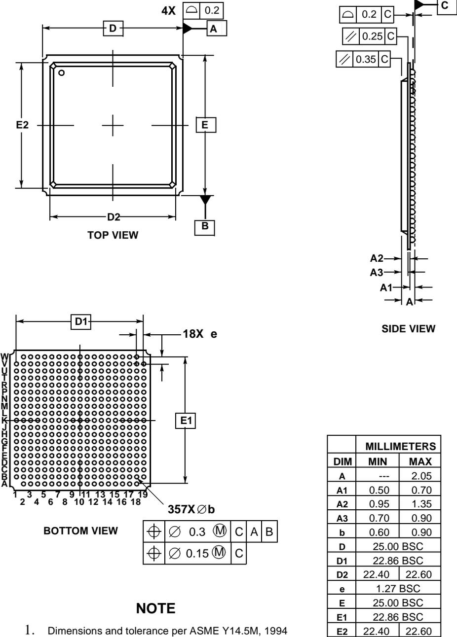
**Figure 76. Mechanical Dimensions and Bottom Surface Nomenclature of the ZP PBGA Package**
