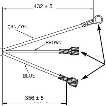
LENGTH IS MEASURED FROM END OF JACKET TO END OF CONDUCTOR BEFORE TERMINAL IS APPLIED.
