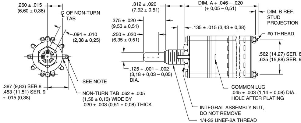
**Note:** Common location for a single pole per deck switch. For common location on multi-pole switches, see circuit diagrams.
