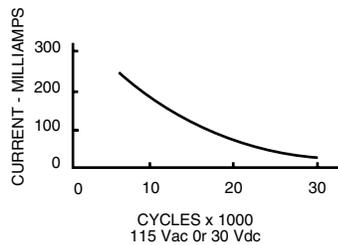
One cycle is 360° rotation clockwise and 360° return. The data for the curve was measured at sea level, 25°C and 68% relative humidity with the life limiting criteria which follows.
