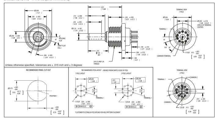
Recommended Mounting Torque: Tighten mounting hex nut to 12 in-lb (15 in-lb max). Before applying torque, rotation of the switch housing must be constrained by the housing flat via the "Recommended Panel Cut-Out" or similar method. Constraining by PCB or anything soldered to the terminals will result in damage to the switch
